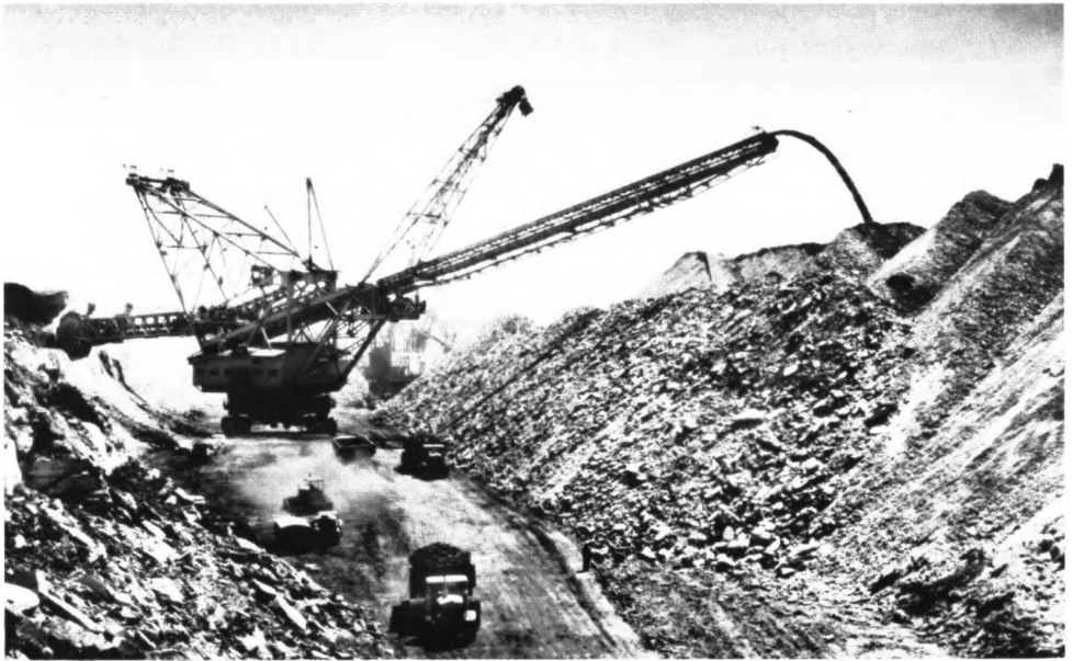
47 Lignite, or brown coal, being mined in Poland with a machine that digs the coal and moves it along a conveyor belt to waiting trucks all in one operation
